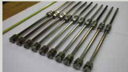
*Pd-based membranes sealed and ready to be integrated in the FERRET prototype.*
