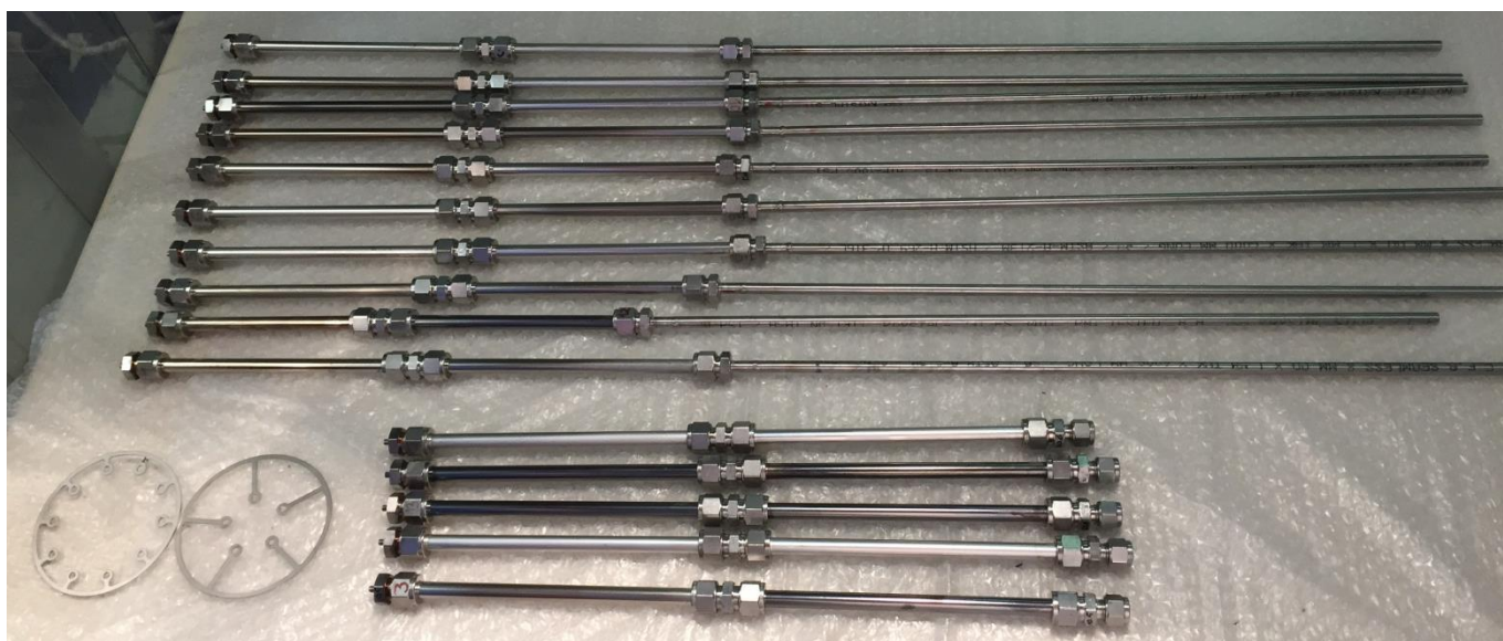
Figure 3. Sealed double membranes before being integrated in the prototype membrane reactor.
